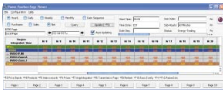
Power position page displaying, by hour, the net total trading position at NYISO.
